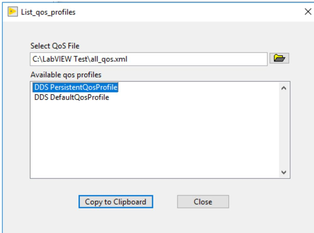
3. In your VI, create a String constant and press Ctrl + V. Connect this String constant to the DDS VI **qos\_profile** terminal. Set the **qos\_uri** as a LabVIEW control or constant and navigate to the path of the QoS Provider file.
