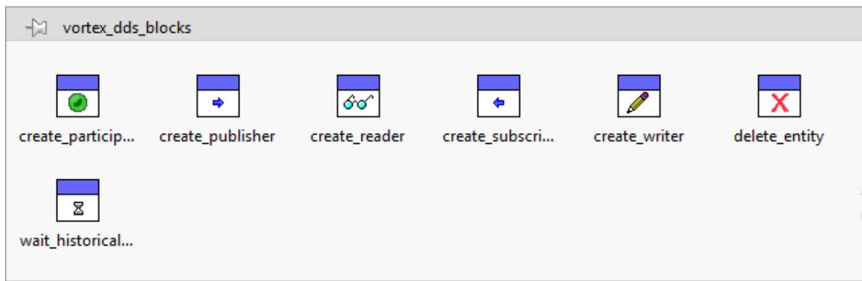
The Vortex DDS LabVIEW VIs are included in **VortexDDS** functions palette.
