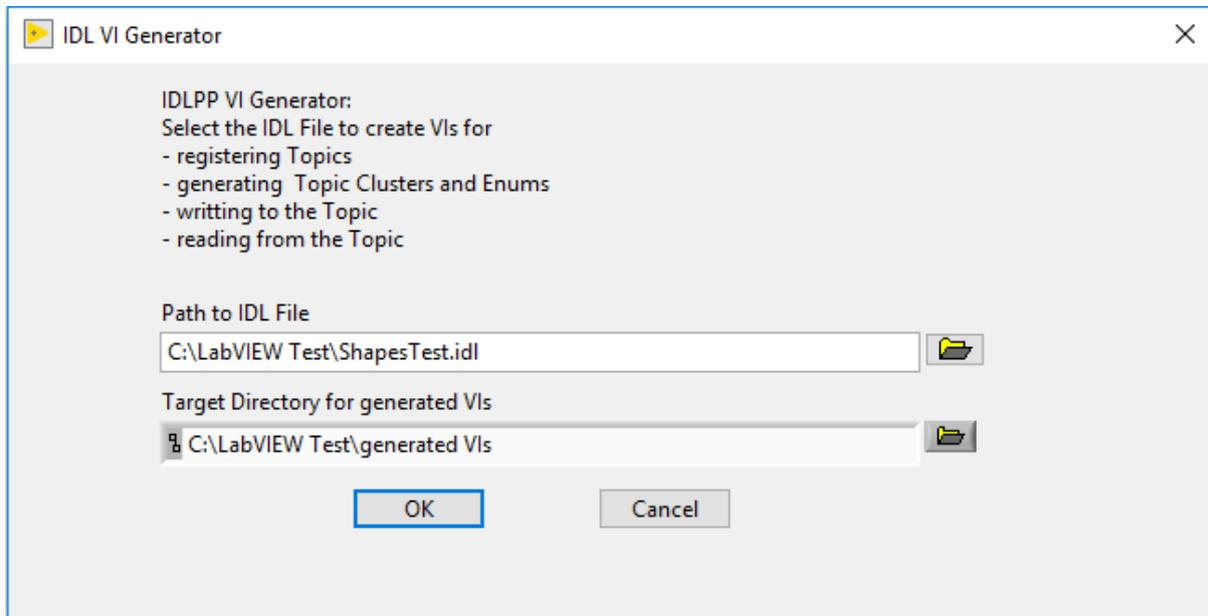
Upon successful generation the VIs are located in the folder that was chosen. A dialog box appears indicating the path of the generated VIs and the IDL file.
