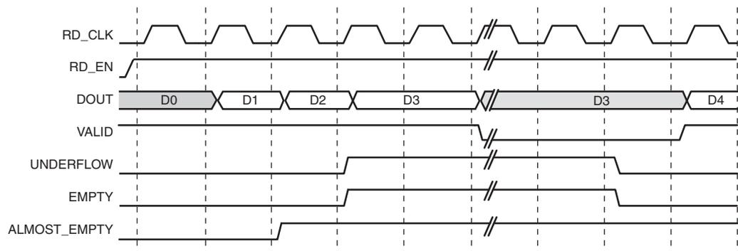
Figure 4-22: FWFT Read Operation for a Synchronous Built-in FIFO with User Embedded Registers Enabled
