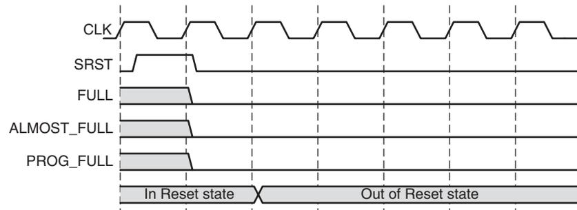
Figure 4-29: Synchronous Reset: FIFO with a Common Clock
