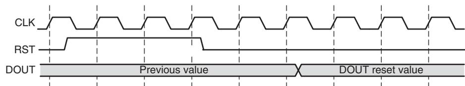
Figure 4-23: DOUT Reset Value for Virtex-6 Common Clock Built-in FIFO Embedded Register
