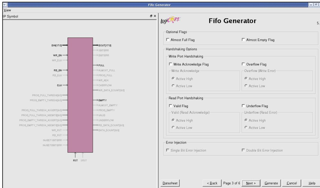
Figure 3-3: Optional Flags, Handshaking, and Initialization Options Screen
