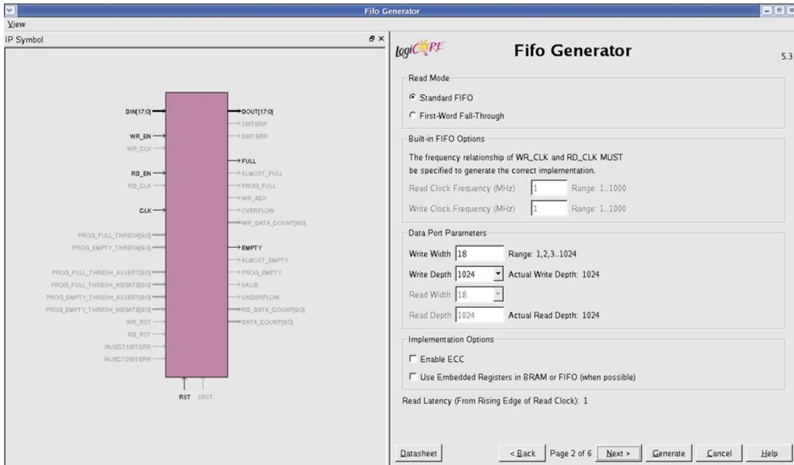
Figure 3-2: Performance Options and Data Port Parameters Screen
