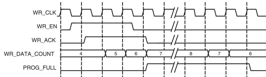
Figure 4-12: Programmable Full Single Threshold: Threshold Set to 7
